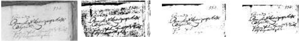
Figure 3. Image1 – From left to right: a. ColorToGray; b. Niblack; c. Otsu; d. Kittler
