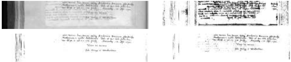
Figure 5. Image2 – From left to right, up to bottom: a. ColorToGray; b. Niblack; c. Otsu; d. Kittler
