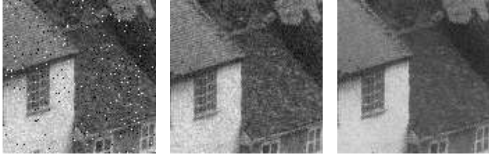
Figure 4. From left to right: a. Image affected by salt and pepper and Gaussian noise; b. Image filtered without salt and pepper noise filter; c. Image filtered using both filtering methods
