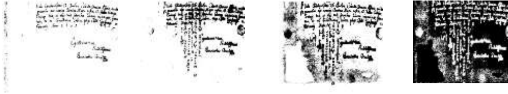
Figure 2. From left to right: a. Otsu Thresholding, b. Kittler Thresholding; c. Niblack Thresholding; d. Sauvola Thresholding
